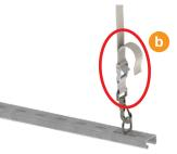
3 Measure 2-3 inches in from where the webbing is hanging down in a straight line and install attachment point hardware (eyebolt, D-Ring)on to the strut bar that will hold the lights.
