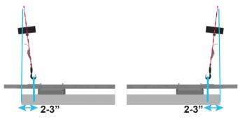
4 Attach the hooks to eyebolts or D-Rings, making sure that there are no twists in webbing and that the excess webbing from the strap is hanging toward the outside of the light bar.
