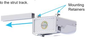
Slide the mounting retainers for the guide pulley into the strut track.
